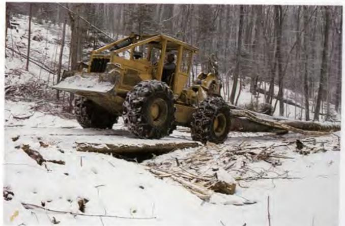
*Portable bridges offer a quicker, less expensive, and much neater alternative to stream crossings than poled fords. When the operation is complete, there is no wood to dispose of, and the bridge is reusable for up to five or more years with careful use.*
